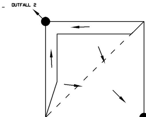
The post-development discharges for Outfall 2 are 3, 6, and 9 cfs for the 2-, 10-, and 100-year design storms, respectively. Outfall 2 meets the peak discharge requirements of the Ordinance because the post-development peak discharges are below the pre-development discharges for Outfall 2.
