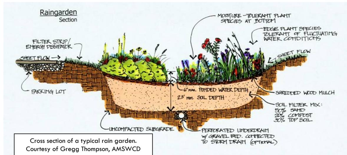
Cross section of a typical rain garden. Courtesy of Gregg Thompson, AMSWCD
